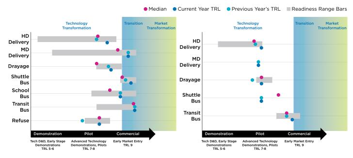
**Figure 4.** Technology readiness level (TRL) across major HDV market segments. Left: (a) on-road battery-electric powertrains. Right: (b) hydrogen fuel cell powertrains. Adopted from California Air Resources Board (2020).
